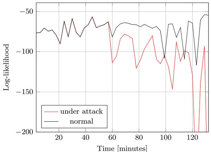
Figure 4: Likelihood values output by the Gaussian-process based model.
