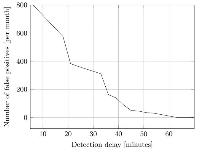
Figure 3: Trade-off between false-positive rate and detection delay.
